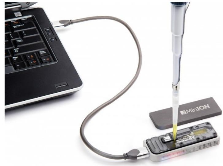
DNA can be sequenced by threading it through a microscopic pore in a membrane. Bases are identified by the way they affect ions flowing through the pore from one side of the membrane to the other.
